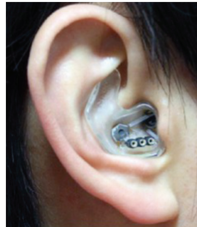
Figure 2. EEG embedded in an earmould. From www.technologyreview.com
