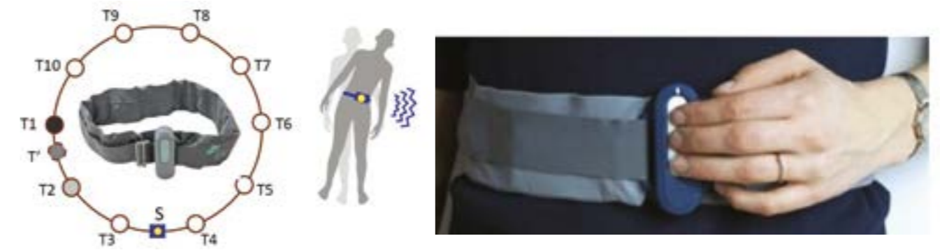
Figure 1: The BalanceBelt provides a vibration pattern around the waist using 10 factors (T1–T10) evenly distributed every 36 degrees. These factors are activated via a microprocessor using a transfer function based on trunk movement and tilt detected by a 6DOF sensor (S). By simultaneously activating two factors at different intensities (linear interpolation), virtually any point around the waist can be stimulated.
